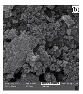
Fig. 2. SEM image of Cu-Co (a) and Cu-Mn (b) mixed oxide
