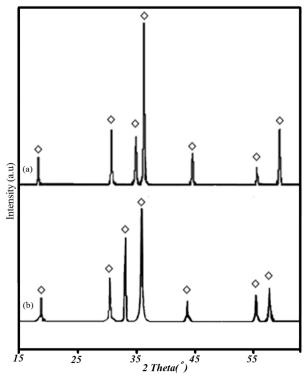
Fig.1. XRD pattern of the Cu-Co (a) and Cu-Mn (b) mixed catalysts
