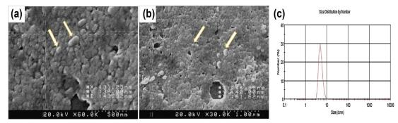
Fig. 13. FESEM image of silver nanoparticles (a) 500 nm and (b) 1  $\mu m$  c) DLS analysis of silver nano particles
