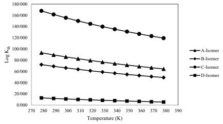
Fig. 4. The effect of temperature on the thermodynamic equilibrium constant (Log  $K_{hh}$ ) values in the temperature range of 278.15-378.15 at 10° intervals.
