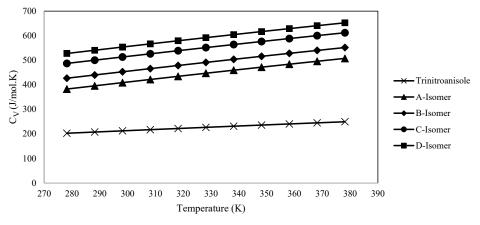
Fig. 5. The effect of temperature on the specific heat capacity  $(C_v)$  values in the temperature range of 278.15-378.15 at 10° intervals.
