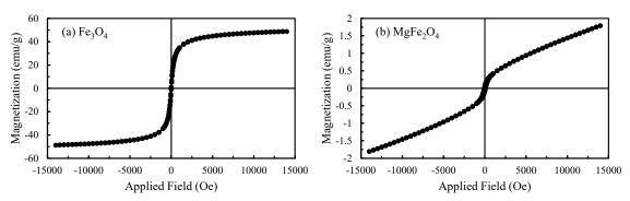
Fig. 4. VSM analyses of Fe<sub>3</sub>O<sub>4</sub> and MgFe<sub>2</sub>O<sub>4</sub> nano adsorbents: (a) Fe<sub>3</sub>O<sub>4</sub>, (b) MgFe<sub>2</sub>O<sub>4</sub>.
