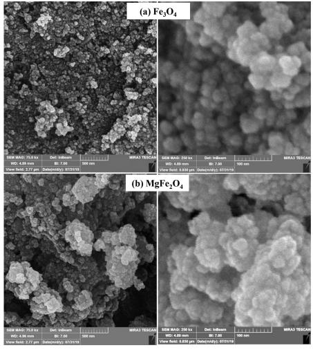
Fig. 2. FESEM images of Fe<sub>3</sub>O<sub>4</sub> and MgFe<sub>2</sub>O<sub>4</sub> nano adsorbents: (a) Fe<sub>3</sub>O<sub>4</sub>, (b) MgFe<sub>2</sub>O<sub>4</sub>.
