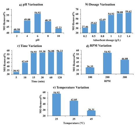
Fig. 7. Effect of adsorption condition variation on adsorption performance of MgFe<sub>2</sub>O<sub>4</sub>
