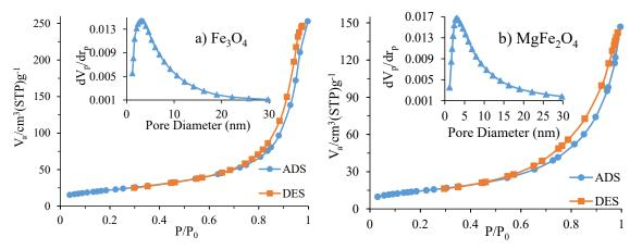
$Fig. 5. Adsorption/Desorption is otherms \ and \ pore \ size \ distribution \ of \ Fe_3O_4 \ and \ MgFe_2O_4 \ nano \ adsorbents: (a) \ Fe_3O_4, (b) \ MgFe_2O_4.$
