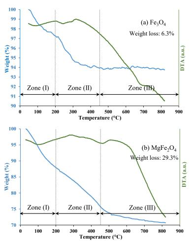
Fig. 6. TG Analyses of Fe<sub>3</sub>O<sub>4</sub> and MgFe<sub>2</sub>O<sub>4</sub> nano adsorbents: (a) Fe<sub>3</sub>O<sub>4</sub>, (b) MgFe<sub>2</sub>O<sub>4</sub>.
