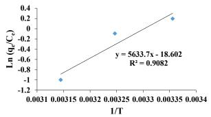
Fig. 8. Curve fitting of the thermodynamic equation for MO adsorption on the MgFe<sub>2</sub>O<sub>4</sub> surface.
