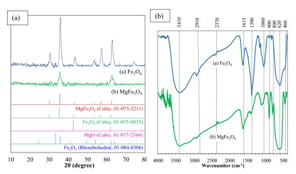
Fig. 1. XRD patterns of Fe<sub>3</sub>O<sub>4</sub> and MgFe<sub>2</sub>O<sub>4</sub> nano adsorbents: (a) Fe<sub>3</sub>O<sub>4</sub>, (b) MgFe<sub>2</sub>O<sub>4</sub>
