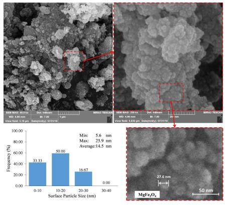
Fig. 3. Surface Particle size distribution histogram of MgFe<sub>2</sub>O<sub>4</sub> nano adsorbents.
