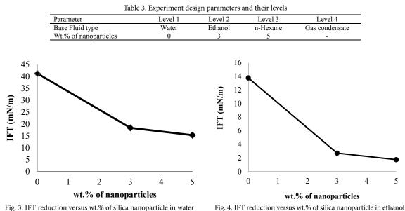
Fig. 3. IFT reduction versus wt.% of silica nanoparticle in water
