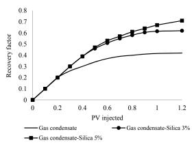
Fig. 11. Oil recovery factor for gas condensate base nanofluids
