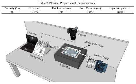
Fig. 2. Schematic of the micromodel Setup
