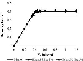
Fig. 9. Oil recovery factor for ethanol base nanofluids
