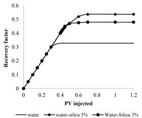
Fig. 8. Oil recovery factor for water base nanofluids
