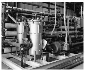
Fig. 7: Reverse osmosis unit at the Flying J Petroleum Refinery [54].
