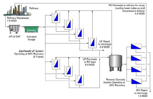
Fig. 13: Wastewater treatment plant in PEMEX refinery, Mexico for reuse purpose [87].
