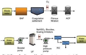
Fig. 10: Process flow diagram of the refinery wastewater reuse system in Sinopec Yanshan Plant [82].
