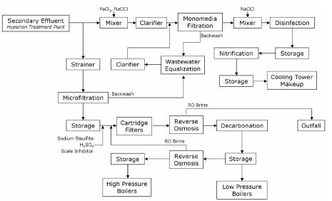
Fig. 5: The process flow diagram of reclamation plant at the Chevron, El Segundo refinery [74].
