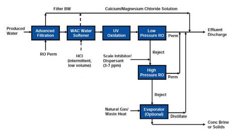
Fig. 14: The process flow diagram of CDM produced water treatment technology [45, 92].
