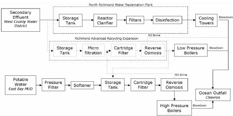
Fig. 6: The process flow diagram of North Richmond Water reclamation Plant and Richmond Advanced Recycling Expansion water project [74].
