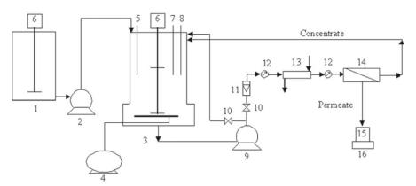
Fig. 2: Schematic of the membrane sequencing batch reactor (MSBR) system applied in Fakhru'l-Razi et al. [20] work (1: raw wastewater tank, 2: peristaltic pump, 3: fermenter, 4: air compressor, 5: pH probe, 6: mixer, 7: temperature probe, 8: DO probe, 9: centrifugal pump, 10: valve, 11: flow meter, 12: pressure gage, 13: heat exchanger, 14: membrane, 15: permeate, and 16: balance) [20].
