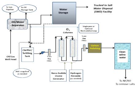
Fig. 15: The pilot system process flow diagram conducted at the #1 Gallo Canyon gas well located approximately 2 miles northeast of Counselors, New Mexico [100].
