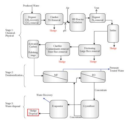
Fig. 12: Newpark Environmental Services produced water treatment system [34, 78].
