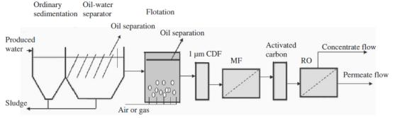
Fig. 3: The schematic diagram of the proposed treatment method for management of produced water at oil production fields by Çakmakce et al. [64].
