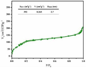
Fig. 3. The N<sub>2</sub> adsorption-desorption isotherm of SH-SiO<sub>2</sub>
