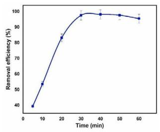
Fig. 8. The influence of contact time on the adsorption of Pb (II) ions by mesoporous adsorbent (aqueous solution volume:20 ml, stirring rate: 350 rpm, initial concentration: 50 mg L<sup>-1</sup>, sorbent dosage: 50 mg, pH= 6)
