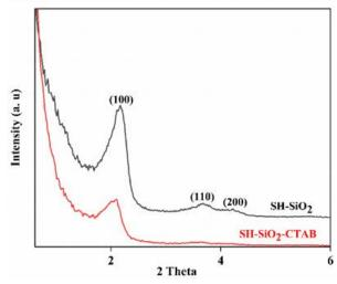
Fig. 1. XRD patterns of  $\mathrm{SH}\text{-}\mathrm{SiO}_{\scriptscriptstyle 2}$  and  $\mathrm{SH}\text{-}\mathrm{SiO}_{\scriptscriptstyle 2}\text{-}\mathrm{CTAB}$
