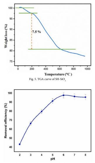
Fig. 6. The effect of solution pH on the adsorption process by mesoporous adsorbent. (aqueous solution volume: 20 ml, striirring rate: 350 rpm, initial concentration: 50 mg. L<sup>-1</sup>, sorbent dosage: 50 mg, contact time: 30 min)
