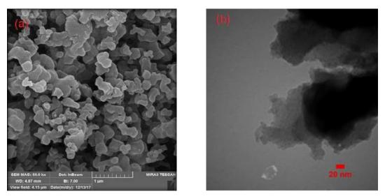
Fig. 2. (a) SEM and (b) TEM image of SH-NPSiO<sub>2</sub>.
