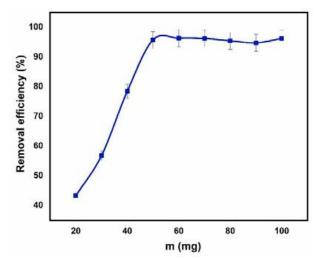
Fig. 7. The effect of adsorbent dose on the adsorption of Pb (II) ions by mesoporous adsorbent (aqueous solution volume:20 ml, striirring rate: 350 rpm, initial concentration: 50 mg. L<sup>-1</sup>, contact tie: 30 min, pH= 6)
