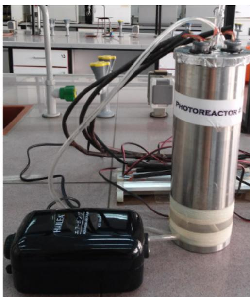
Fig. 1. Photoreactor used in the experiments
