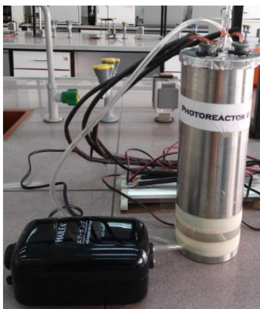
Fig. 1. Photoreactor used in the experiments
