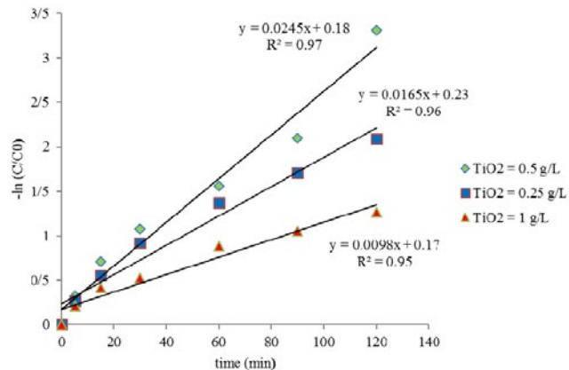
Fig. 7. Effects of  $\text{TiO}_2$  amount on degradation kinetics (CLM=2 g/l, pH=5)
