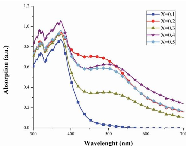
Fig. 3. UV-visible absorption spectra of the Cd<sub>x</sub>Zn<sub>1-x</sub>O composites with different compositions.
