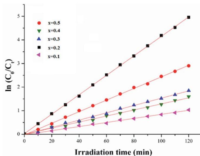
Fig. 7. Variation of  $\ln(C_0/C_t)$  vs. irradiation time under the visible light on the  $Cd_xZn_{1-x}O$  nanocomposites.
