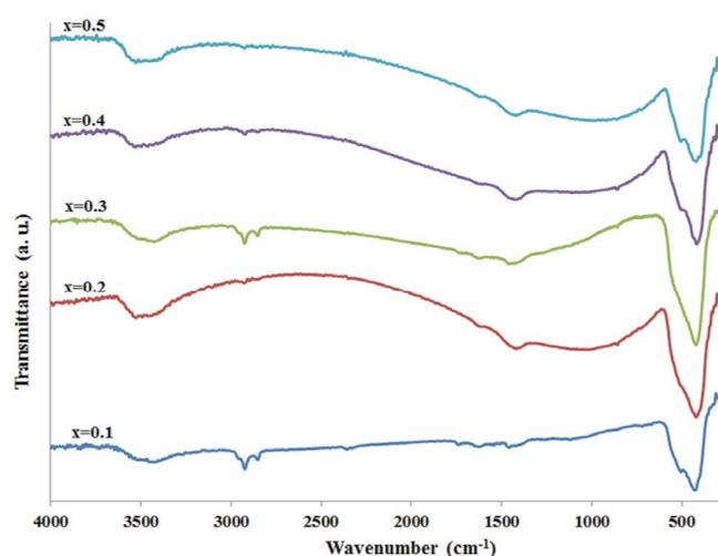
Fig. 6. FT-IR spectra of different CdO-ZnO samples
