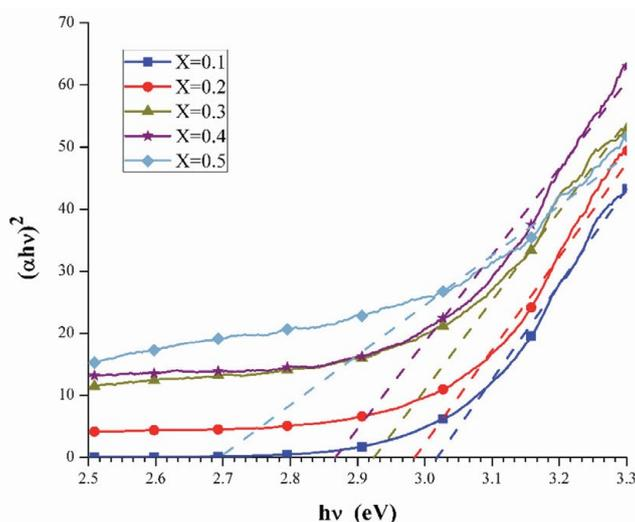
Fig. 4. The Tauc plot of different CdO–ZnO samples
