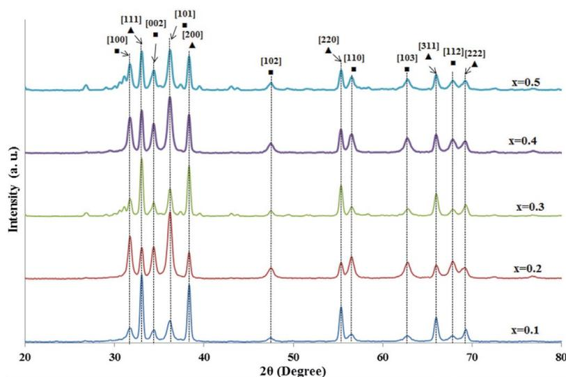
Fig. 2. X-ray diffraction pattern of different-ZnO samples
