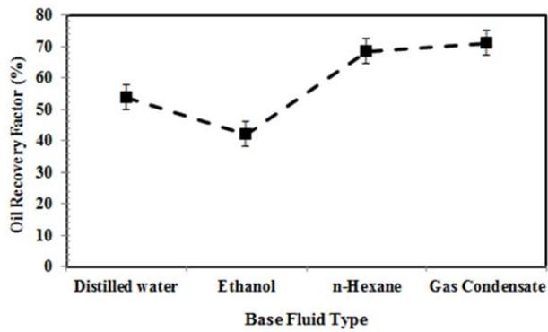
Fig. 15. Effect of the base fluid type on the oil recovery
