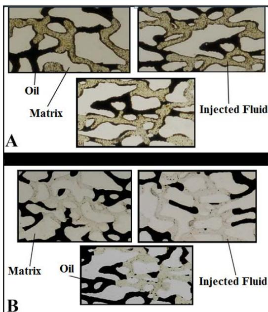
Fig. 12. Pore scale photos of different parts of micromodel glass: A) water injection and B) water-silica injection
