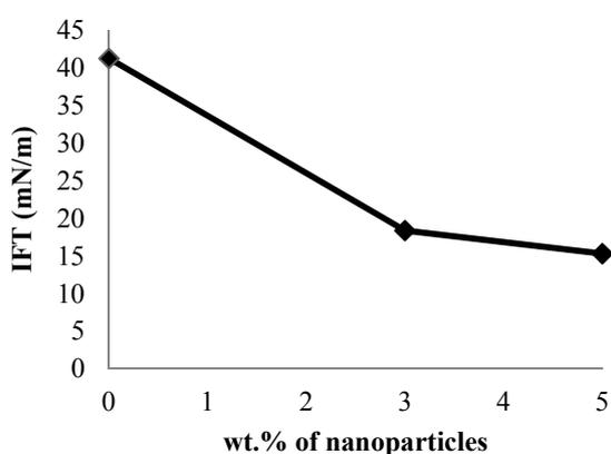
Fig. 3. IFT reduction versus wt.% of silica nanoparticle in water
