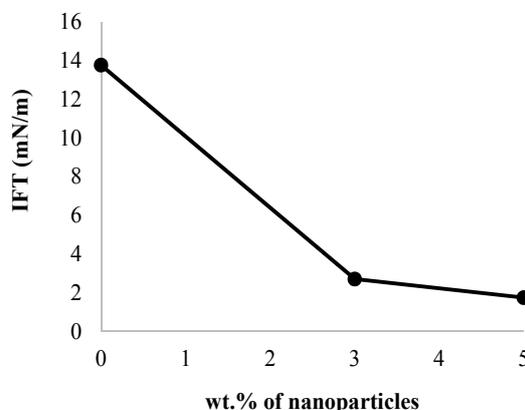
Fig. 4. IFT reduction versus wt.% of silica nanoparticle in ethanol
