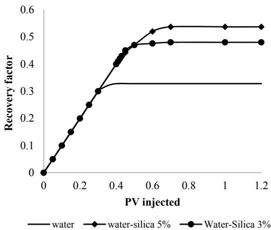
Fig. 8. Oil recovery factor for water base nanofluids
