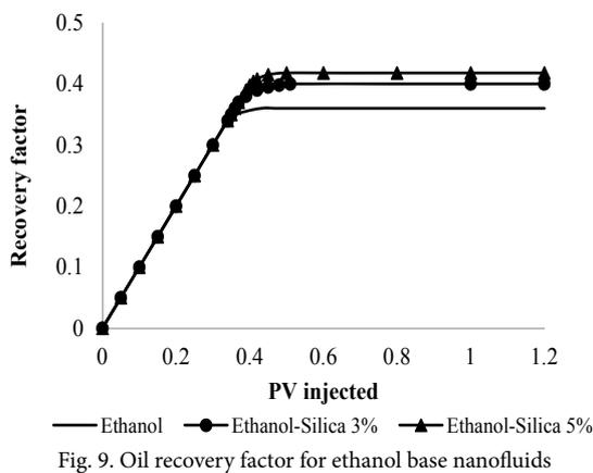
Fig. 9. Oil recovery factor for ethanol base nanofluids
