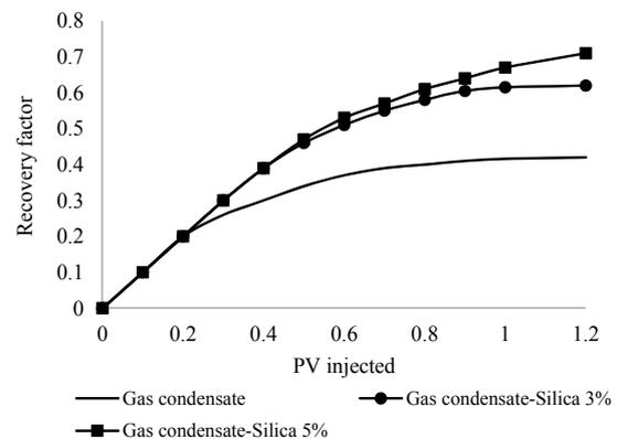
Fig. 11. Oil recovery factor for gas condensate base nanofluids
