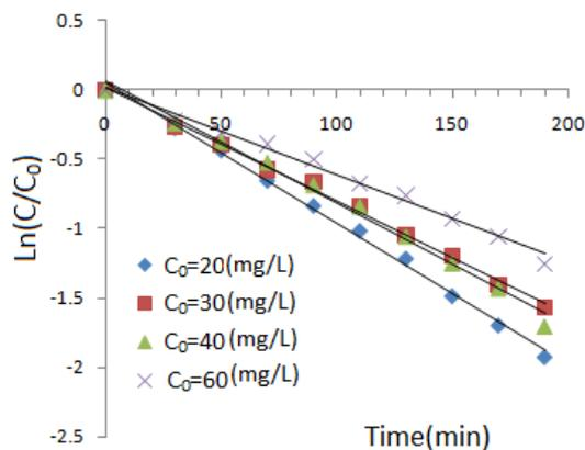
Fig. 9: Effect of initial concentration on the degradation of 2,4-DCP. Irradiation. source: visible lamp, 100mL 2,4-DCP, 10mg catalyst
