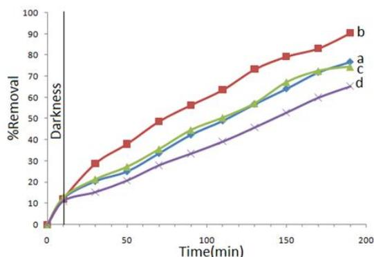
Fig. 8: Photocatalytic removal of 2,4-DCP over a) MWCNTs/ Co-TiO<sub>2</sub> (3.03), b) MWCNTs/ Co-TiO<sub>2</sub> (3.13), c) MWCNTs/ Co-TiO<sub>2</sub> (3.52) and d) MWCNTs/ Co-TiO<sub>2</sub> (4.14) (2,4-DCP Conc. 40 mg/L, 10 mg catalyst, 100 mL 2,4-DCP, visible light, irradiation time: 180 min and H<sub>2</sub>O<sub>2</sub> conc. 0.01M).
