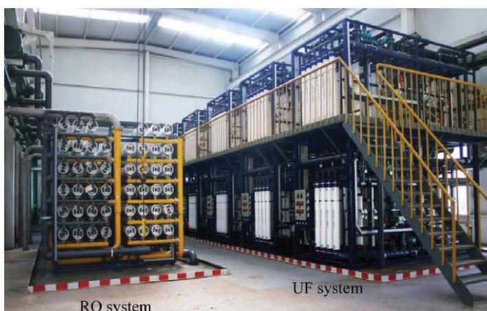
Fig. 11: RO and UF systems in Sinopec Yanshan Plant [82].
