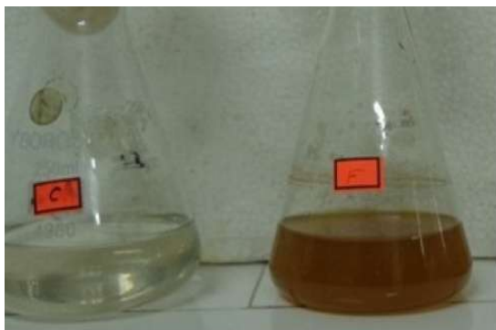
Fig. 1. Biosynthesis of silver nanoparticles by Fusarium solani showing colour change from colourless to brown colour
