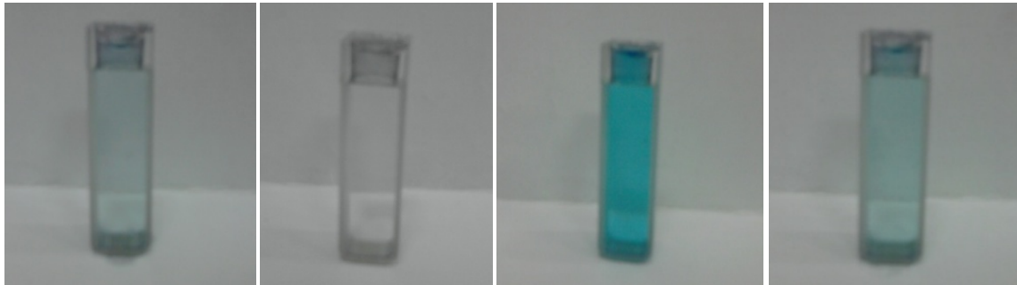
Fig. 14. From left to right, the color of the sample before being put under solar light, after 15, 25 and 50 min under solar light, respectively.
